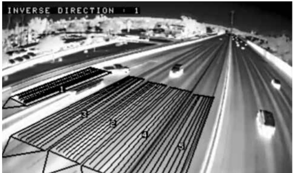
Thermal imaging cameras pick up heat coming off the environment and are therefore the ideal tool to detect vehicles on highways or on highway ramps.
